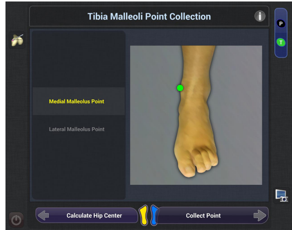
Figure 17. Collect the medial and lateral malleoli points to calculate the ankle center.
