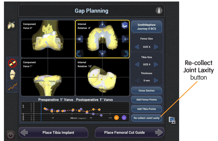
Figure 46 Press the Re-collect Joint Laxity button to access the Joint Laxity – Extension screen.
