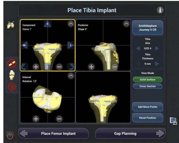
Figure 41. Tibial prosthesis placement in Solid Surface view.
